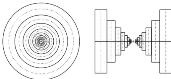
**Figure:** Disk ring structure as adopted for our calculations. The radius of the rings increases exponentially.
