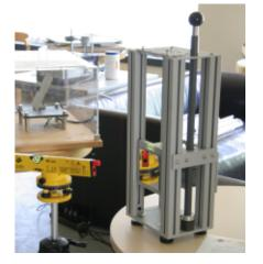
Mirrors in terrestrial gravitational wave detectors must be shielded against seismic noise, i.e. ground movements. This is achieved by suspending them like pendulums, with a sharply defined resonance frequency far from the actual frequency range of the detector. However, the mirrors may then be excited to rather large oscillations at the resonance frequency, making the detector as a whole unstable. To counteract this, the oscillations can be damped using eddy current damping.
