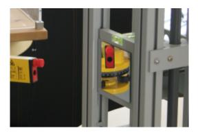
This working model demonstrates a suspended mirror equipped with an eddy current damping which can be activated or deactivated by a mechanical lever. A laser beam reflected from the mirror serves to reveal the movements more clearly. The mirror can be made to move in different ways, allowing the observation of the effect of the eddy current damping on the different modes of motion.
